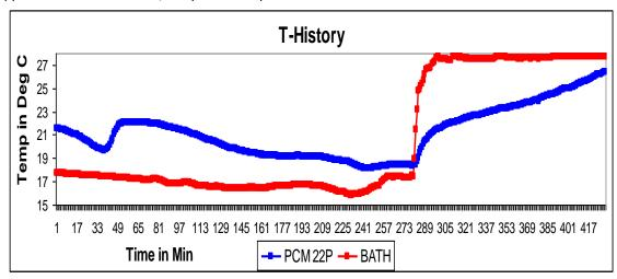
30g sample is taken in a test tube in molten condition and placed in a temperature controlled bath. A temperature sensor is placed in the test tube and bath to record the temperatures using a data logger. The bath is maintained at around 17  $^{0}$ C during the freezing cycle and at around 27  $^{0}$ C during the melting cycle.
